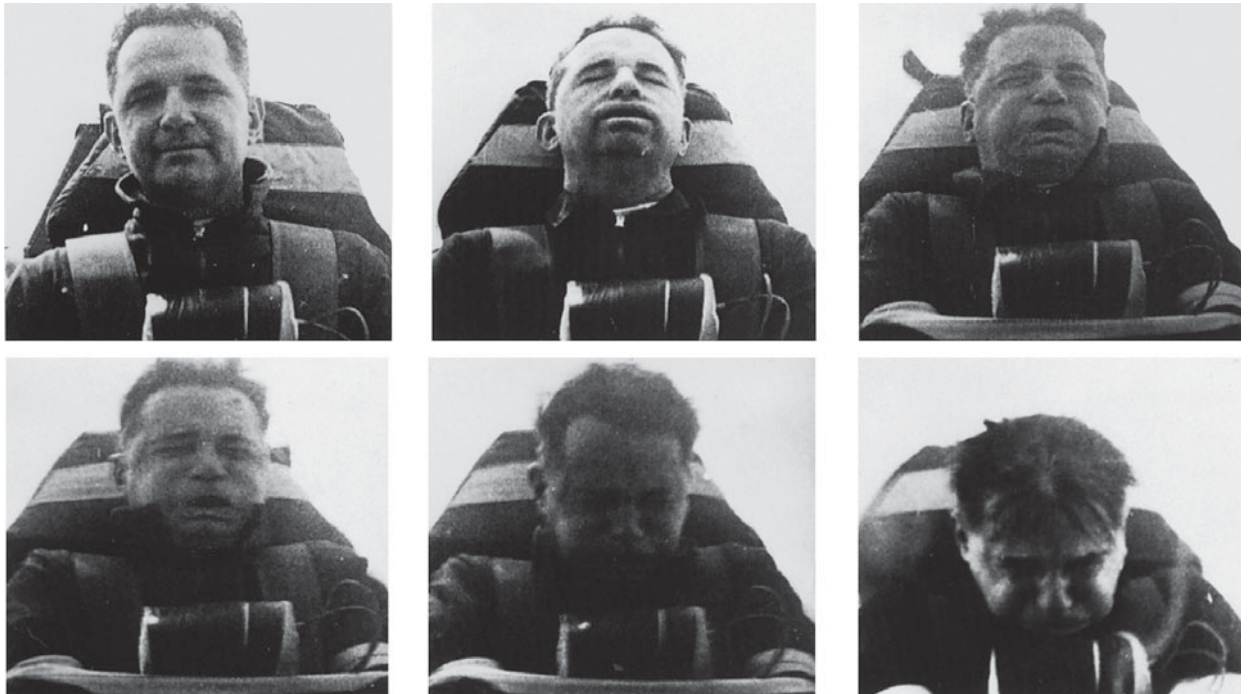
Figure 2-7 Colonel J. P. Stapp in a rocket sled as it is brought up to high speed (acceleration out of the page) and then very rapidly braked (acceleration into the page).
